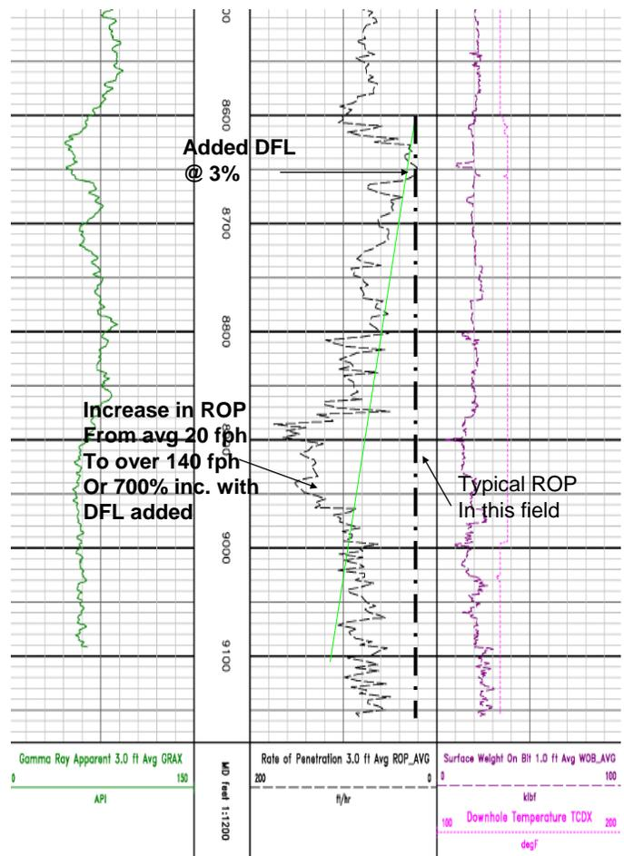
DFL into the system promoted wellbore stability thus allowing the operator eliminate post-drilling reaming in preparation for the production casing run. All tolled, this resulted in an overall operational efficiency improvement of over 30%, thus surpassing the operator’s expectations for economic viability. The DFL has now been incorporated as a standard technology on all of their wells since.
